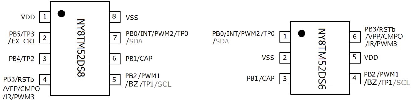
Figure 1 Package pin assignment
